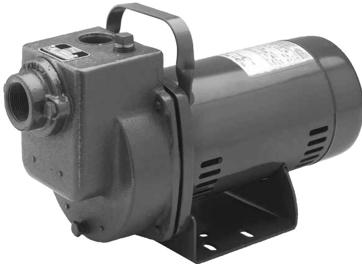
The DPC Series self-priming centrifugal pump is a rugged cast iron pump capable of priming up to 20' vertically and will handle solids up to 0.225" diameter. The unit is equipped with a 1/2 HP 115-volt motor and features 1-1/4" suction and discharge.
